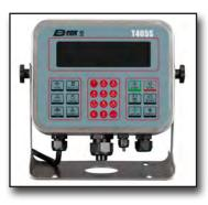
T405S Programmable Selections: Same as T403S plus Eight-Point Linearization • 2 Serial Ports with full duplex Operational Keys: Same as T403S plus alpha-numeric, common symbols Display: Same as T403S
