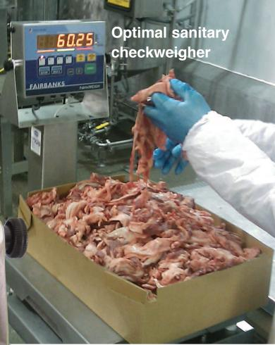
While the NexWeigh is versatile enough for use in a variety of applications, it is ultimately a premium checkweighing instrument due to its sanitary design, commercial approval, IP69K washdown rating and easy-to-use front panel checkweighing functions.
