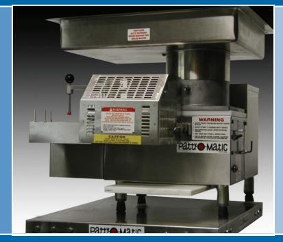
Height: 28" Depth: 30" Width: 28" Volts: 115 standard/220 available Motor: 1/2 H.P. Amps: 13 Weight: 225 lbs Cycle: 60 standard/ 50 available Production: 1800-2100 per hour Mold Plate: up to 3/4" thickness in any shape
